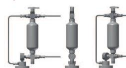
The ability to purge the sample point ensures optimal retrieval of a representative, contamination free sample. The S23 type sampler provides a system purge in addition to a fixed sample volume. No vent connection is needed. The vent is connected to the top valve. This way a loop is created in order to fill the bottle by means of gravity.
