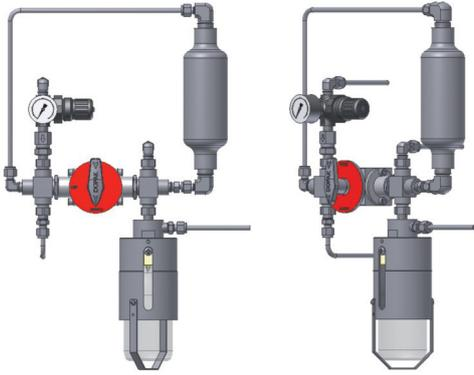
The ability to purge the sample point ensures optimal retrieval of a representative, contamination free sample. The S32 type sampler provides a system purge and needle purge in addition to a fixed sample. The unique design offers a one handle operation by multiple valves, allowing for sampling independent of the process conditions. These features provide sample accuracy and safety.
